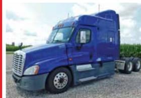
**2012 Freightliner Cascadia**, 64" mid-roof sleeper, Cummins ISX, 450 hp, Eaton 10 spd., airliner air ride suspension, power windows, locks, mirrors, tilt wheel, air ride driver's seat, cruise control, diff lock, stationary 5th wheel, dual 120 gal. alum. fuel tanks, 228" wheel base, 22.5 LP tires, (6) alum. wheels, VIN 1FUJGLB4CSBN1505
