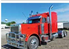
**2003 Peterbilt 379 Ex. Hood**, 63" standup sleeper, Caterpillar C-15 Acert, 550 hp, Eaton 18 spd., 1850 torque, DS 404 rear ends, 3.55 ration, diff lock, flex leaf susp., dual 135 gal. alum. fuel tanks, dual 8" straight pipes, dual step boxes, dual Vortex 15" cleaners, 18" Texas bumper w/ deer guard, stainless steel 1/4 fenders, stainless steel lightbars, AC, power right window, heated mirrors, sliding 5th wheel, susp. dump valve, dual air ride seats, (10) alum. wheels, VIN 1XP5DB9X43D805386
