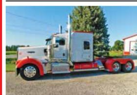
**2005 Kenworth W900L**, flat top sleeper, 72" aerodynamic, C15 Acert, Cat 550 hp, twin turbo, Eaton 13 spd., Eaton rear ends 3.36 ratio, AG200 8 bag susp. w/ updated swing arms, dual 15" air cleaners, dual 8" straight pipes, dual step boxes, dual 120 gal. fuel tanks, 18" frame mount step box, stainless steel light bar & lights, stainless air box
