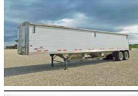
**2018 Timple**, hopper bottom, 45'Lx96"Wx78"H aluminum, Shurlock roll tarp, commodity doors, (8) alum. wheels, 2 spd. landing gear, 2 spd. hopper doors, alum. sub-frame front & rear, (8) 24.5 LP tires (NEW), VIN 1TDDH40021JB159253
