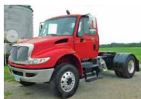
**2012 International 4300 Durastar**, 103,000 miles, air ride day cab, Maxi Force DT, 245 hp, Allison Auto, rear end 20K diff. lock, tilt wheel, heated mirrors, air ride suspension, 70 gal. fuel tank, dual air ride seats, AC, cruise control, VIN 3HCMMMAAN1CL665389
