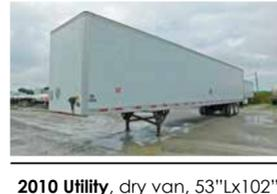
**2011 Utility**, dry van, 53"Lx102"Wx110"H alum. roof, food grade liner, logistic posts, 2 spd. landing gear, 22.5 LP tires, steer wheels, VIN 1UYYS2533BP121504
