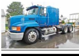
**1994 Mack CH600**, 40" sit down sleeper, Mack E6, 350 hp, Eaton Super 10, Mack air ride susp., air slide 5th wheel, dual 120 gal. fuel tanks, tilt, AC, cruise control, dual air ride seats, 11R 24.5 tires, (6) alum. wheels, VIN 1M1AA13Y4RW039192
