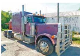
**2004 Peterbilt 379 Ex. Hood**, 1,082,550 miles, 63" standup bunk, Caterpillar C-15, single turbo, 550 hp, Eaton 18 spd, RTLO18918B Eaton DS 404, 3.55 ratio, diff lock, flex leaf air ride susp., eng. brake, Texas bumper, dual vortex, air cleaners, dual exhaust, dual 135 gal. alum. fuel tanks, power steering, tilt wheel, AC, cruise control, stainless steel lightbars, OH at 805,000, 24.5 LP tires, (1) alum. wheels VIN 1XP5DB9X34D827090
