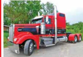
**2005 Kenworth W900L**, Aerodyne sleeper, Caterpillar C-15 Acert, 550 hp, Eaton 13 spd., Eaton rear ends, 3.25 ratio, diff lock, dual exhaust, dual air cleaners, Jones performance hood w/ W900A lights, air slide non-grease 5th wheel, full double-hump fenders, dual air ride seats, AC, power windows, cruise control, engine brake, (2) beds, 22.5 tires, (10) alum. wheels, VIN 1XKWDB9X35V052917 (1 year left on platinum overhaul warranty)
