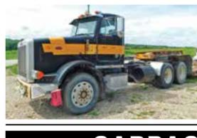
**1989 Peterbilt 378**, day cab, Caterpillar 3406 B ATA, Eaton 13 spd., Peterbilt 4 bag air ride susp., Eaton rear ends, 2 line wet kit, single 100 gal. fuel tank, single exhaust, 24.5 tires, (10) alum. wheels, VIN 1XPFD89X4KN276437
