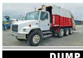
**1994 Freightliner FL80**, garbage truck, Cummins 8.3 hp., Allison automatic, Dayton 10x20 drive tires, 11R22.5 tag, 10x20 steer tires, VIN 1FUXJLBB3RL626895
