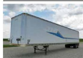
**1996 Trailmobile**, dry van, 53'x13'6" translucent roof, 110" door opening, plywood lined, alum. scuff plate, threshold plate, 2 spd. landing gear, sliding tandem, air ride susp., 22.5 LP tires, steel budd wheels, VIN 1PT01JAH3T9008181
