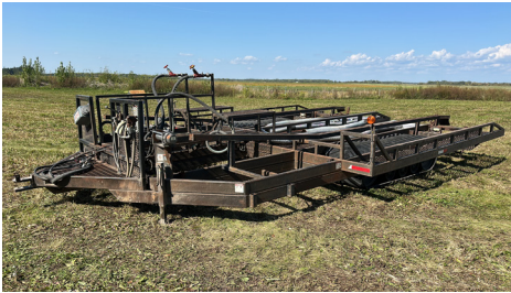
Shop built NH3 double tank trailer
